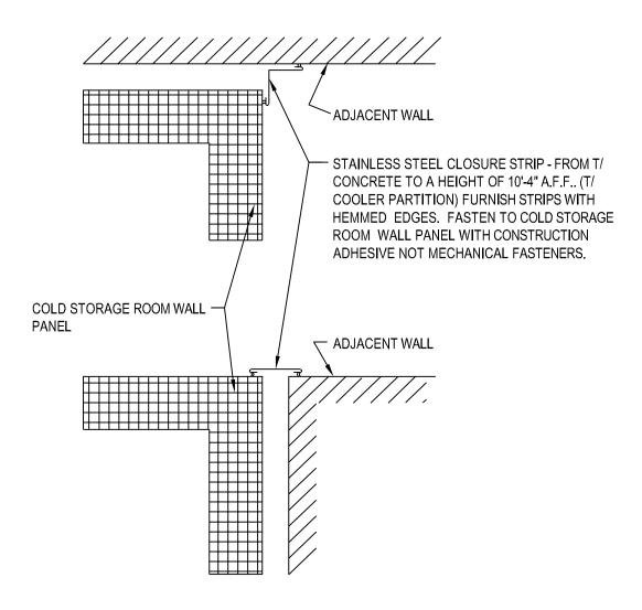
DESIGN COLD STORAGE ROOMS WITH MINIMUM 2" WIDE AIR SPACE BETWEEN COLD STORAGE ROOM WALL PANELS AND ADJACENT WALL SURFACES. WHEN COLD STORAGE ROOM IS LOCATED ADJACENT TO EXTERIOR WALL OF BUILDING, CONSIDER INCREASING WIDTH OF AIR SPACE.
